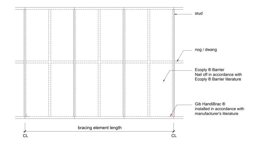
Figure 1e: Bracing Panel Installation - Long
