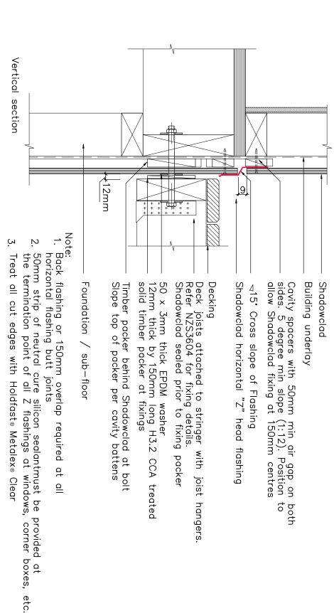
SC048: Shadowclad@Mid Floor to Non—Cantilevered Deck (Cavity)
