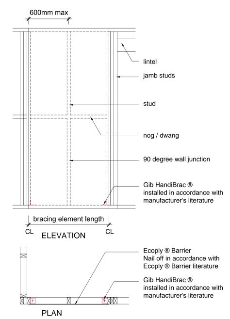
Figure 1f: Bracing Panel Installation at Lintel
