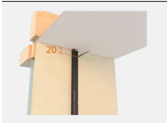
Figure 14: 20 mm end distance
