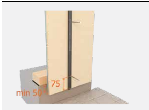
Figure 13: 75 mm end distance
