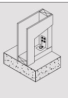
Position GIB HandiBrac® as close as practicable to the internal edge of the bottom plate.
