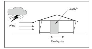
Ecoply structural plywood is manufactured to AS/NZS 2269, and it is suitable for design and use in earthquake and wind bracing systems constructed in accordance with NZS 3603 and AS/NZS 1170.
