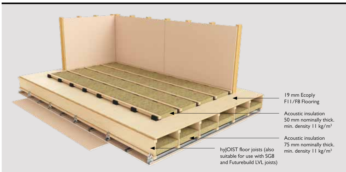
Figure 8: Insulation Requirements
