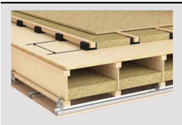
Figure 4: Acoustic cradles Spacing Along the Length of the Batten
