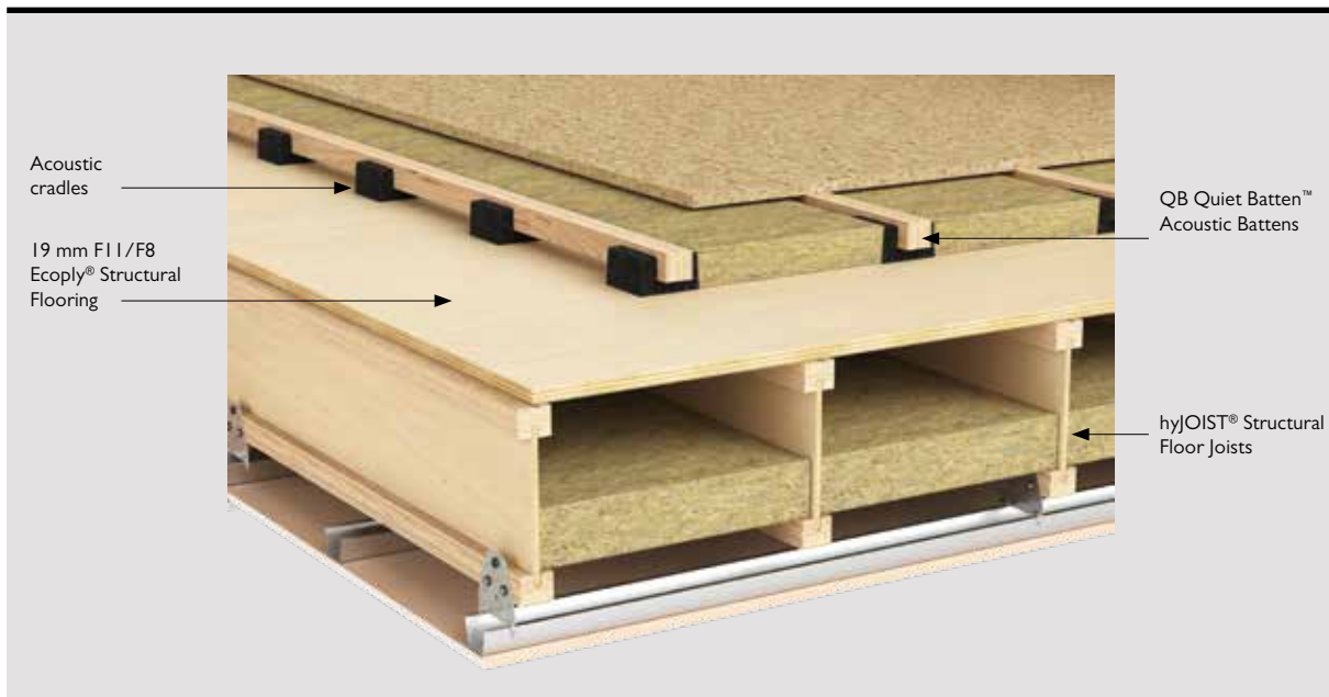
Figure 1: Typical Batten & Cradle™ Flooring System
