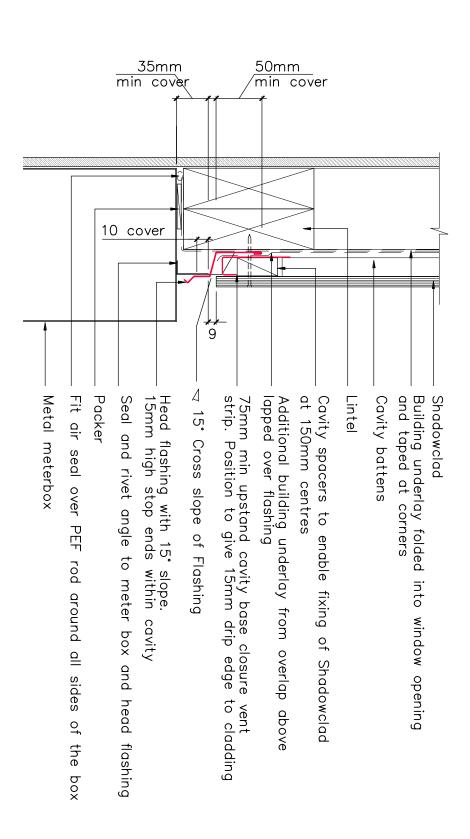
SC034A: Shadowclad@Meterbox Vertical Cross Section (Cavity)
