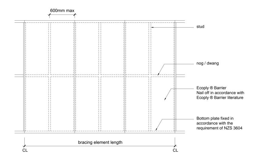
Figure 1g: EPBS Bracing Panel Installation
