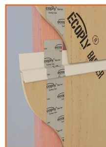
Ecoply sealing tape extends under the horizontal 'Z' flashing or the Ecoply Barrier 150 mm Frame Sealing Tape on to the framing
